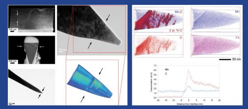
Analysis by atom probe tomography reveals the austeniteferrite interface, and the distribution of alloying elements in the material. Segregation can be visualized in 3D, and mapped over planar or complex interfaces to produce composition profiles.
