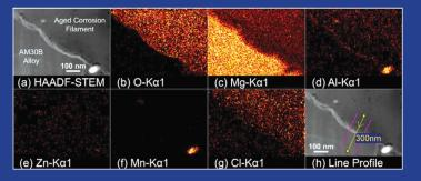
STEM image of aged corrosion filament and (b)-(g) corresponding EDS maps for O, Mg, Al, Zn, Mn and Cl across the filament/alloy interface.
