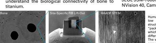
Human bone investigated at two length scales. The low magnification SEM image (a) shows bone structural units, osteons, which are mineralized "packets" of bone. (b) A FIB lift out from an osteon, which can be imaged using (c) HAADF STEM, where different orientations of collagen can be revealed. The white arrow points to longitudinal and the black arrow points to transverse collagen orientations.
